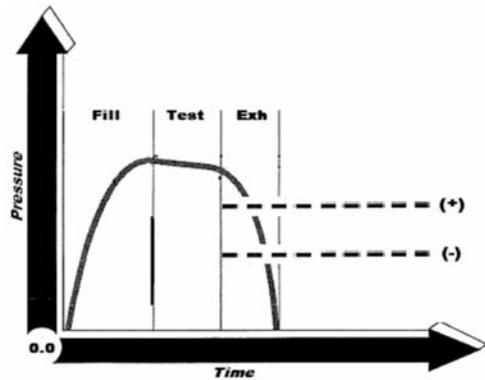
The figure to the right shows a typical back-pressure flow test in which the part passes the evaluation. In this example, the residual back-pressure seen at the part's inlet (while the outlet is vented to atmosphere) was within the established reject minimum and reject maximum limits, indicating that the passage was the correct size.
