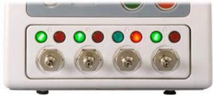
A red fail light indicates that at least one test parameter went out of tolerance at some time during a test cycle. The fail light turns on if a gross leak occurred, a pressure error value is exceeded, or the product exceeded an established pressure or flow tolerance. Repeated failures can indicate Sprint iQ or external fixtures have set-up problems.
