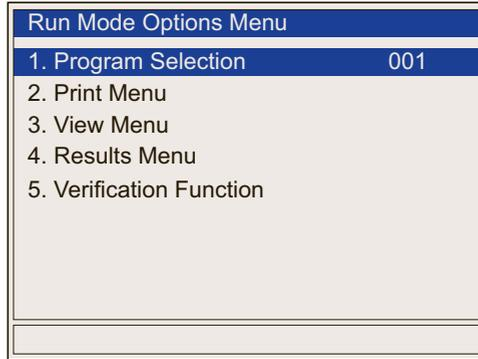
Use the **Up** and **Down** keys to highlight the option name and press **Enter** to select. For example, press **Enter** when Program Selection is highlighted and the “Parameter Editor” will appear (as seen on page 27). The “Parameter Editor” permits easily changing values by using the arrow keys.
