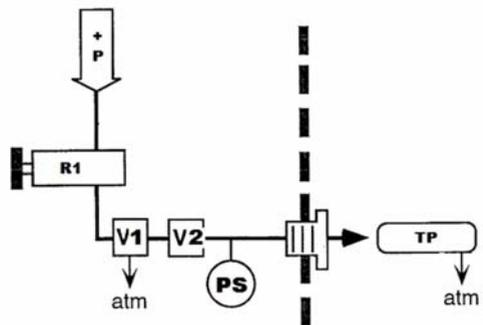
2. Part is pressurized with positive pressure [+P] to the desired test pressure set by the pressure regulator [R1] by opening valves [V1] and [V2] throughout the test.
