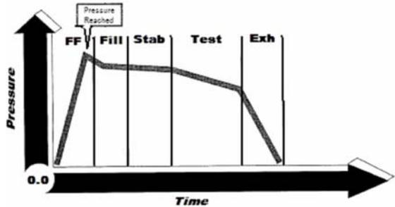
pressure higher than the actual leak test pressure. This higher pressure fills the test part faster (equivalent to a Fast Fill). After this step is completed, the first program links to the actual test program with the target test pressure.
