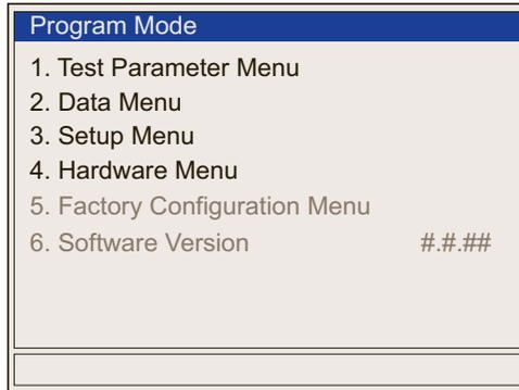
Highlight the first item, Test Parameter Menu, and press **Enter**. The Test Parameter Menu will open and the display will appear as shown below. The navigation method is similar in all menus.
