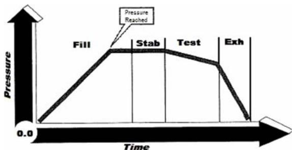
over time. The Electronic Programmable Regulator automatically adjusts to achieve the target test pressure.
